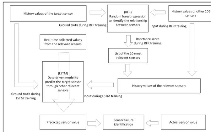
Figure 1. The process of sensor failure identification based on RFR-LSTM
