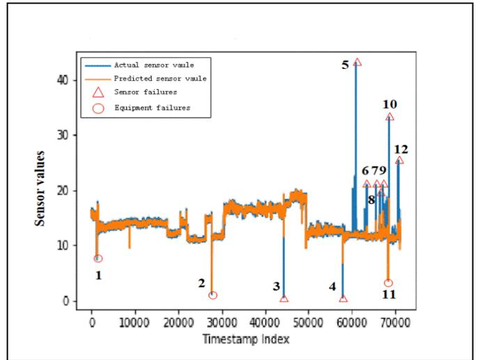
Figure 4. Identified sensor failures according to the difference between the predicted and actual sensor values
