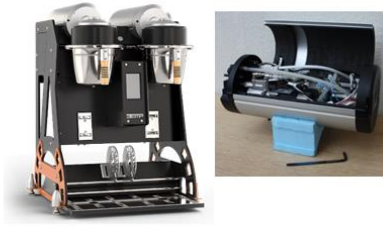
Figure 11 – Repair: 3Temp coffee machine designed for easy access and maintenance with one tool
