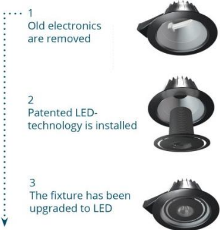
Figure 8 – Upgrading: New LED solutions on the existing fixture, reference: https://www.fischer-lighting.com/english/
